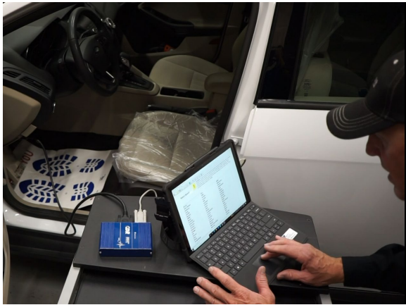
Figure 1: Nederveld technician performing imaging of vehicle ACM.
