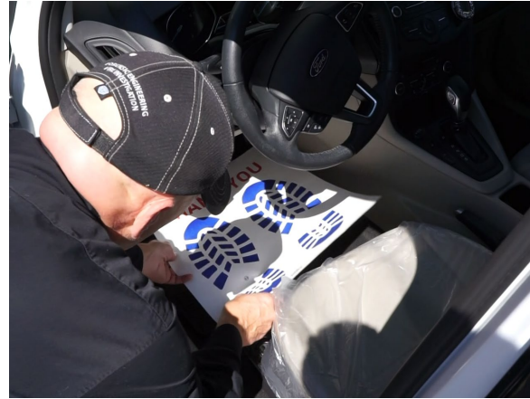
Figure 5: Technician places seat covers and floor mats to protect vehicle interior.
